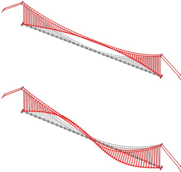
According to the considerations presented above, a set of eigenmodes under permanent loading was calculated for the bridge. The first two modes are shown in Fig. 9. Based on this set of basis functions, the buffeting analysis was performed for a wind profile where the mean wind is given by a logarithmic distribution and the power spectral density is of Kaimal type.
