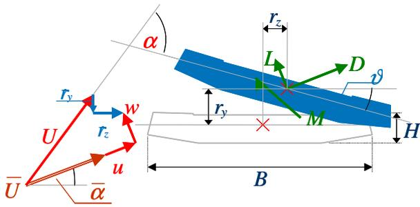
This situation is indicated in Fig. 5. The overall effective wind velocity and incident angle results from a vectorial addition of the single velocity components. For evaluating the forces according to Eq. (4), only a linearization is applied.
