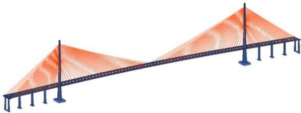
reduction of 3D to 2D is in general applicable, because one dimension – the main span, or the height of the pylons – of a structural part is dominant with respect to the other two dimensions, cf. Fig. 2 for the Stonecutters bridge. Since the structural analysis is based on a modal approach, the air flow can be adequately described by characterizing the wind forces for fixed cross sections and certain type of movement.
