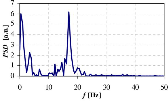
By considering the power spectrum of the time history, cf. Fig. 4, often pronounced peaks at non-zero frequencies are observed. The most dominant peak indicates the vortex shedding frequency. It is expressed in a non-dimensional manner by the Strouhal number
