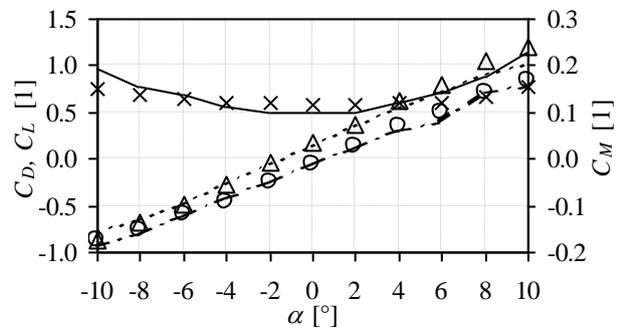
*Fig. 2.* Steady state coefficients of Hardanger bridge deck:  $C_D$  (x),  $C_L$  (o) and  $C_M$  (Δ)
