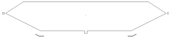
Fig. 3. Cross section with wind guiding vanes and spoiler for Hardanger bridge.
