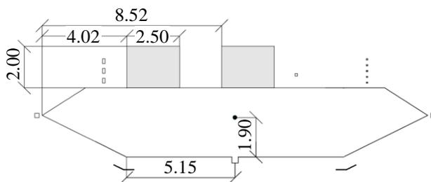
Fig. 7. Cross section for traffic calculation.
