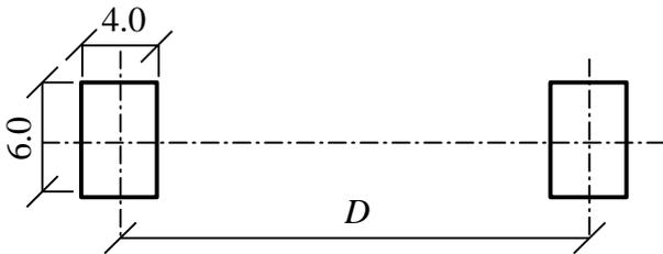
*Fig. 9.* Cross section model for pylon investigations.
