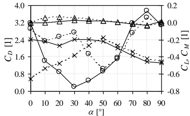
*Fig. 10.* Steady state coefficients  $C_D$  (x),  $C_L$  (O) and  $C_M$  ( $\Delta$ ) for left (solid) and right (dashed) pylon leg.
