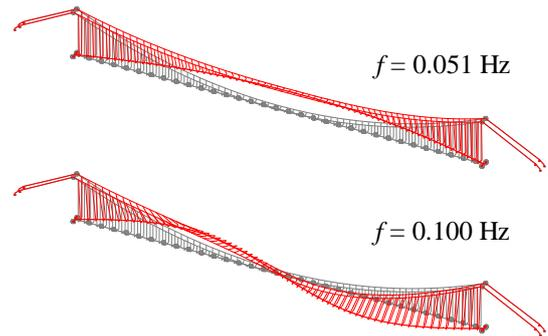
Fig. 14. First two eigenmodes of Hardanger bridge deck.
