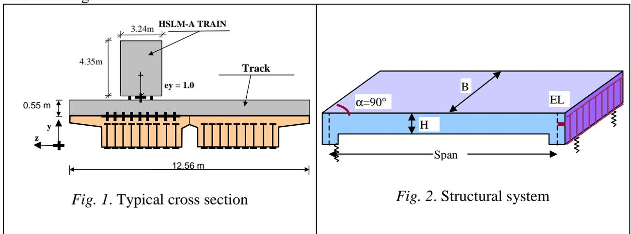
Fig. 1. Typical cross section
