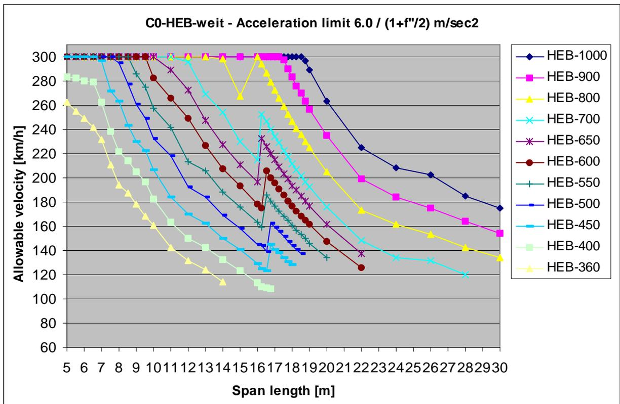
Fig. 6. Allowable travel speeds for existing structures (limit  $6.0 \text{ m/s}^2$ )
