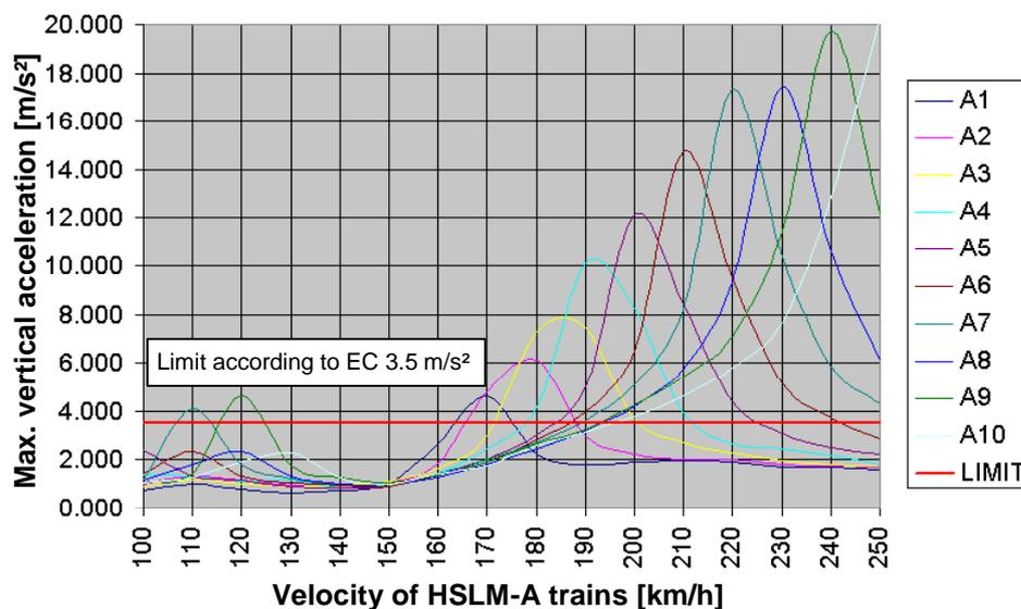
Fig. 3. Maximum vertical acceleration for different trains
