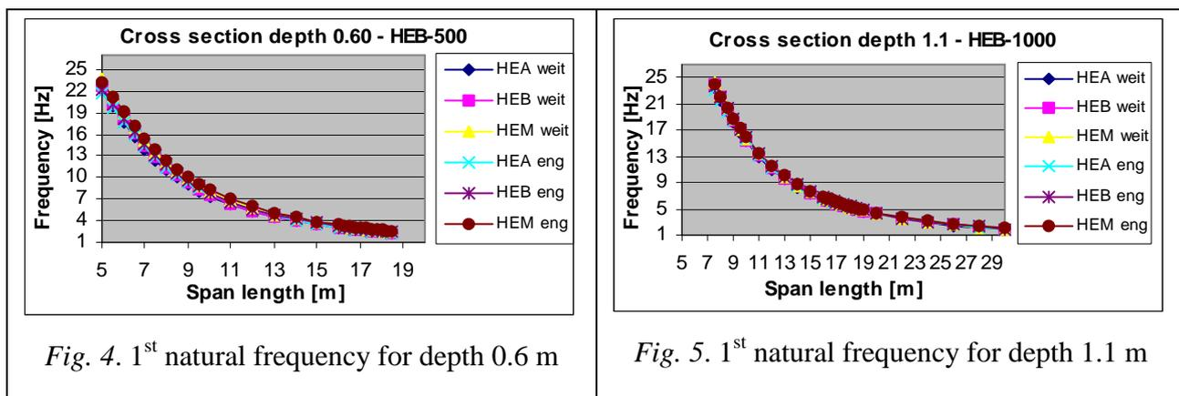
Fig. 4. 1<sup>st</sup> natural frequency for depth 0.6 m
