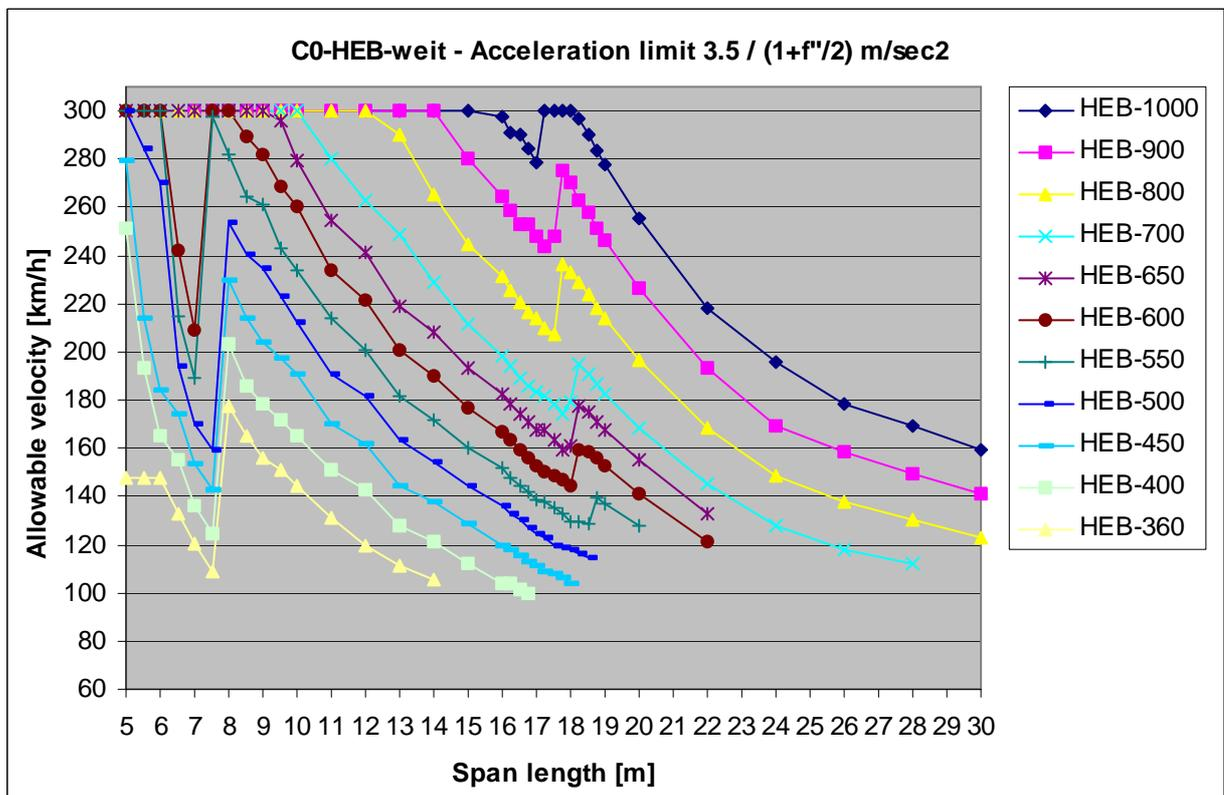
Fig. 7. Allowable travel speeds for new structures (limit  $3.5 \text{ m/s}^2$ )
