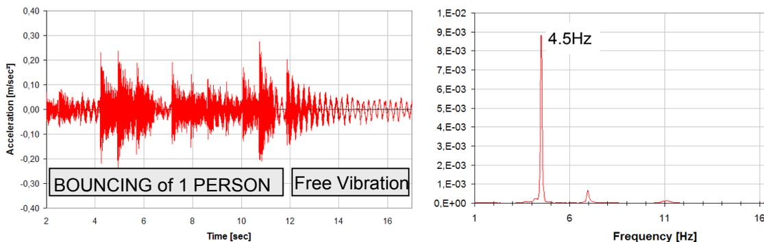
Figure 4. Vertical time-history for 1 person bouncing on bridge #1, 'CF5', and a PSD-spectrum
