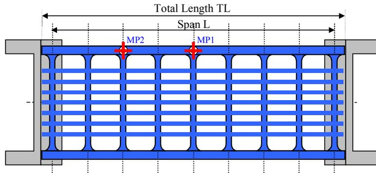
Figure 2. Schematic plan of the investigated bridges including instrument layout
