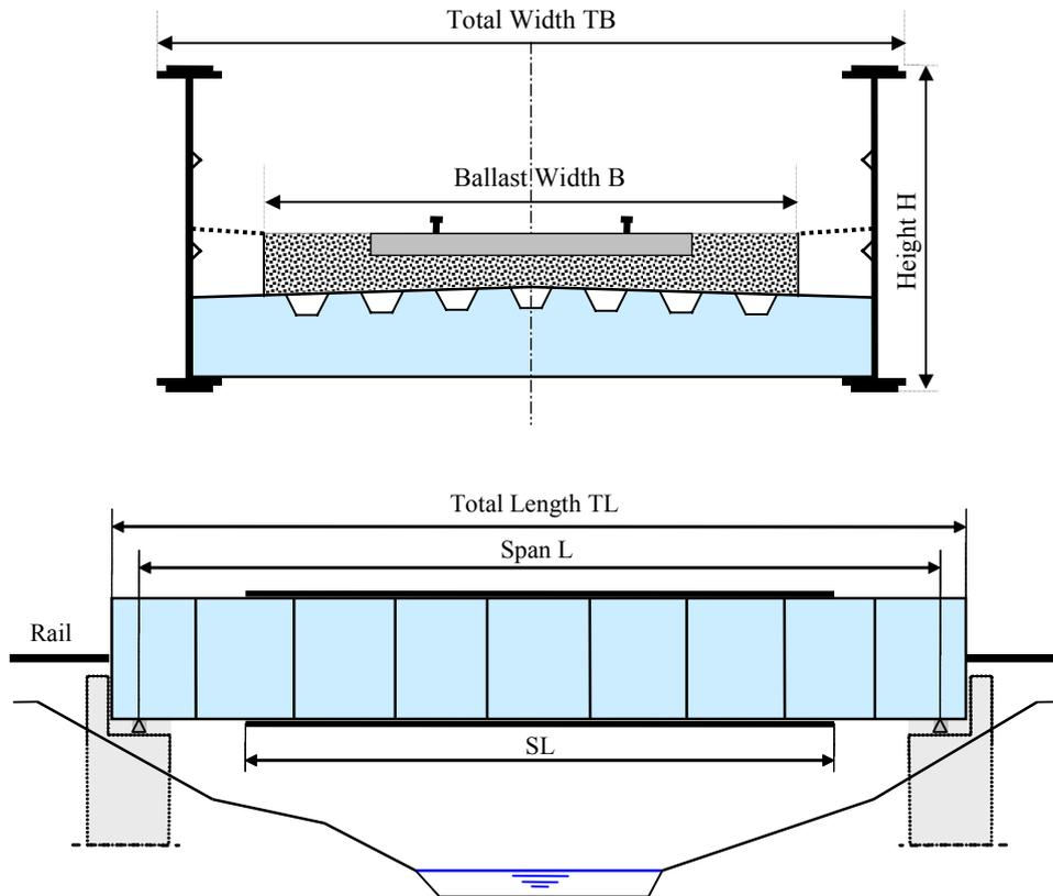
Figure 1. Cross section and elevation of investigated steel bridges
