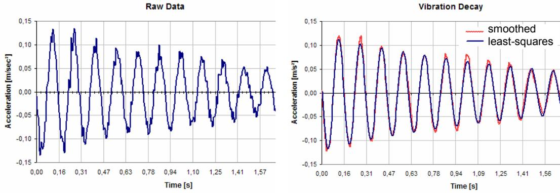
Figure 5. Parameter identification (eigenfrequency, damping.....) for vibration decay
