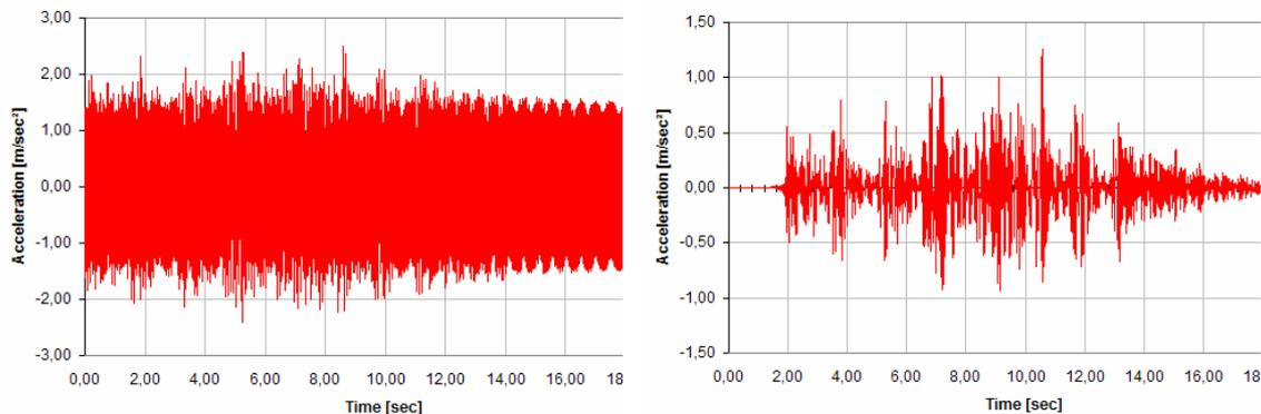
Figure 6. Vibration measurement of bridge #2 with and without ground loop effects.
