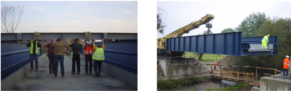
Figure 3. 7 people bouncing on bridge #1, 'CF1' and deck installation of bridge #2
